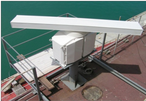
Photo 2. The NEVA-type Radar. Photo by TETIS Integrated Systems LTD
