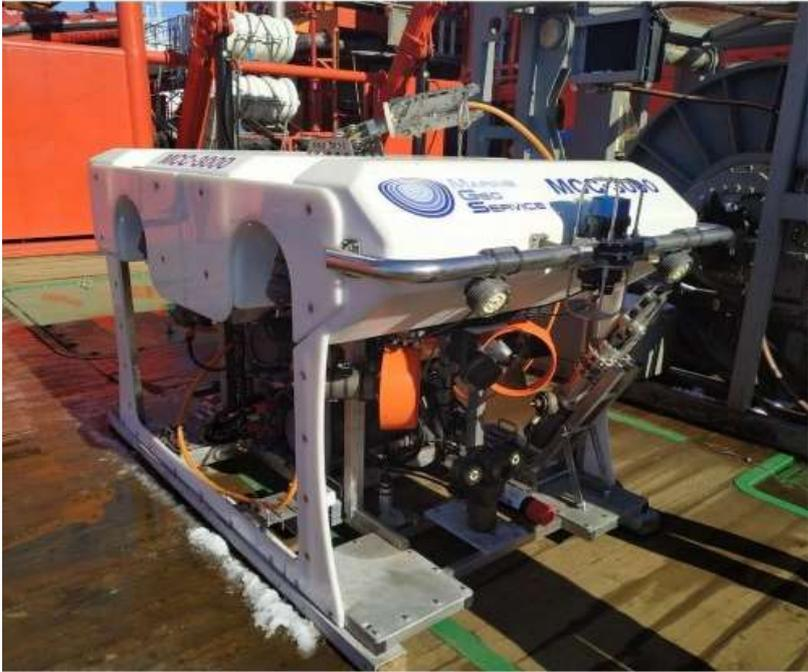
MSS-3000 remotely operated underwater vehicle.
