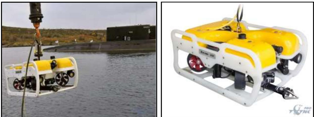
The Marlin-350 unmanned remotely operated vehicle (ROV)
