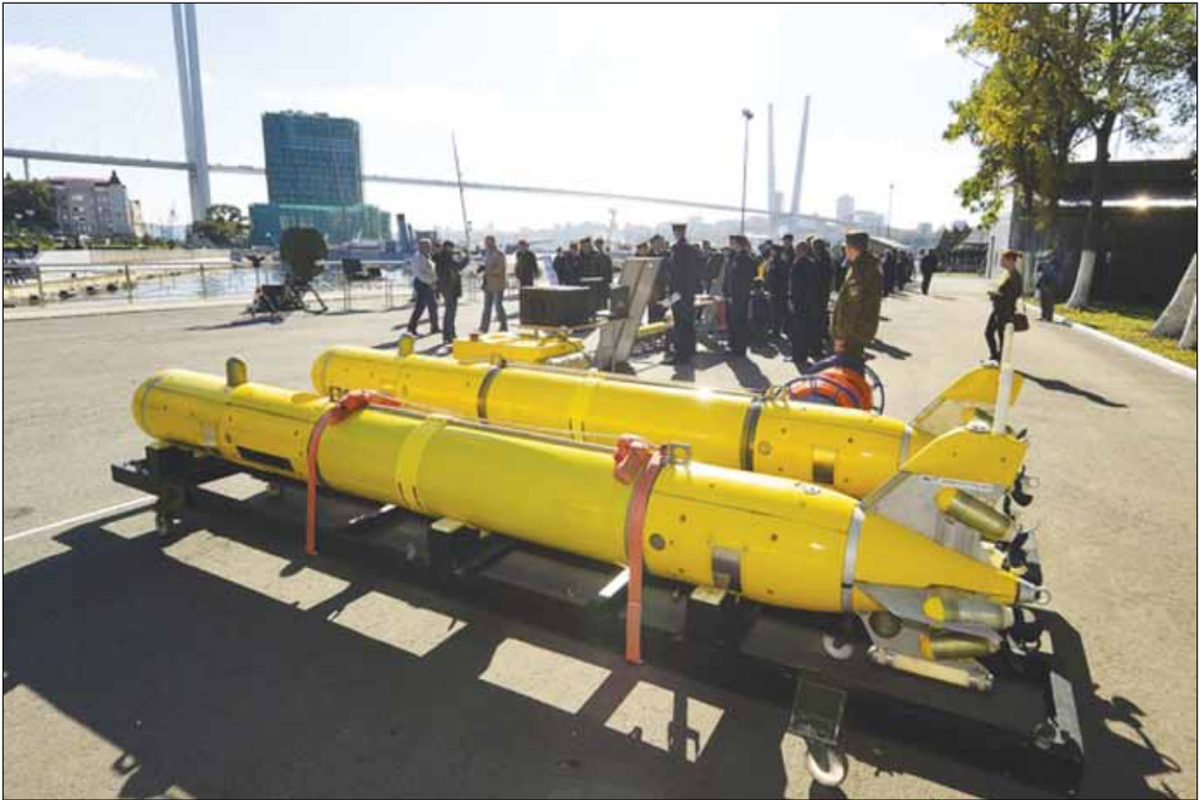
Photo 6. Russian mobile underwater multipurpose complex Galtel-Alevrit. Used in Syria in the Tartus Naval Facility Point of Russia
