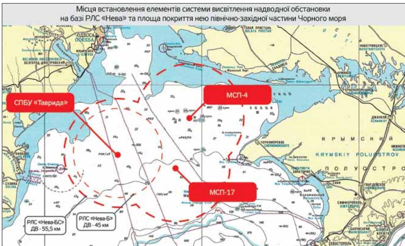
Fig. 2. The places of deployment of the elements of the surveillance system for surface environment on the base of NEVA radar and the coverage range of the north-western part of the Black Sea.
